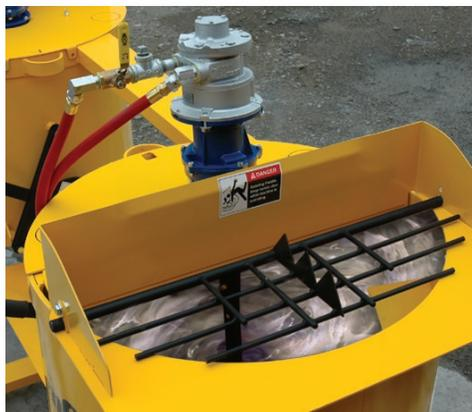
Specially designed mix tank provides high shearing action for thorough and complete particle wetting, producing superior grout.
