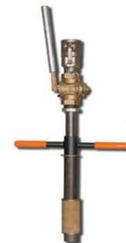
**Mechanical Surface Packer.** Equipped with shut-off valve and a quick disconnect fitting.
