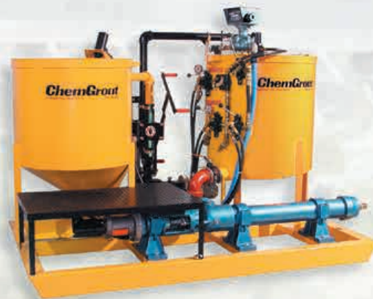
Dual speed 3L8 grout pumps are offered on the CG-680 series. Low speed delivers 20 gpm, high speed 45 gpm.
