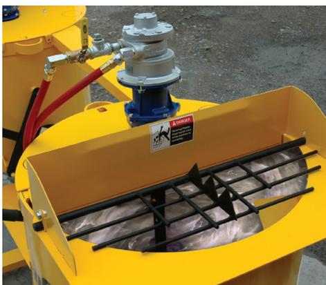
ChemGrout's high-efficiency, variable speed paddles provide reduced mix time, enhancing flow rate and maximizing jobsite operation.
