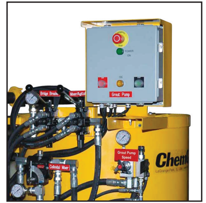
ChemGrout offers both manual and automatic (pictured) pressure controls on the CG680 Series.
