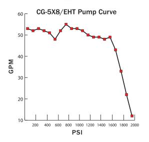
Double-Acting, Positive Displacement, Plunger Pump
